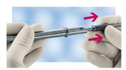
Pull inner tube out of outer shaft.
