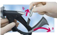
Remove CO<sub>2</sub> cylinder from handle.
